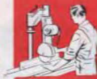
Blade is pulled through lumber . . . weight of swing arm returns blade to retract position.
