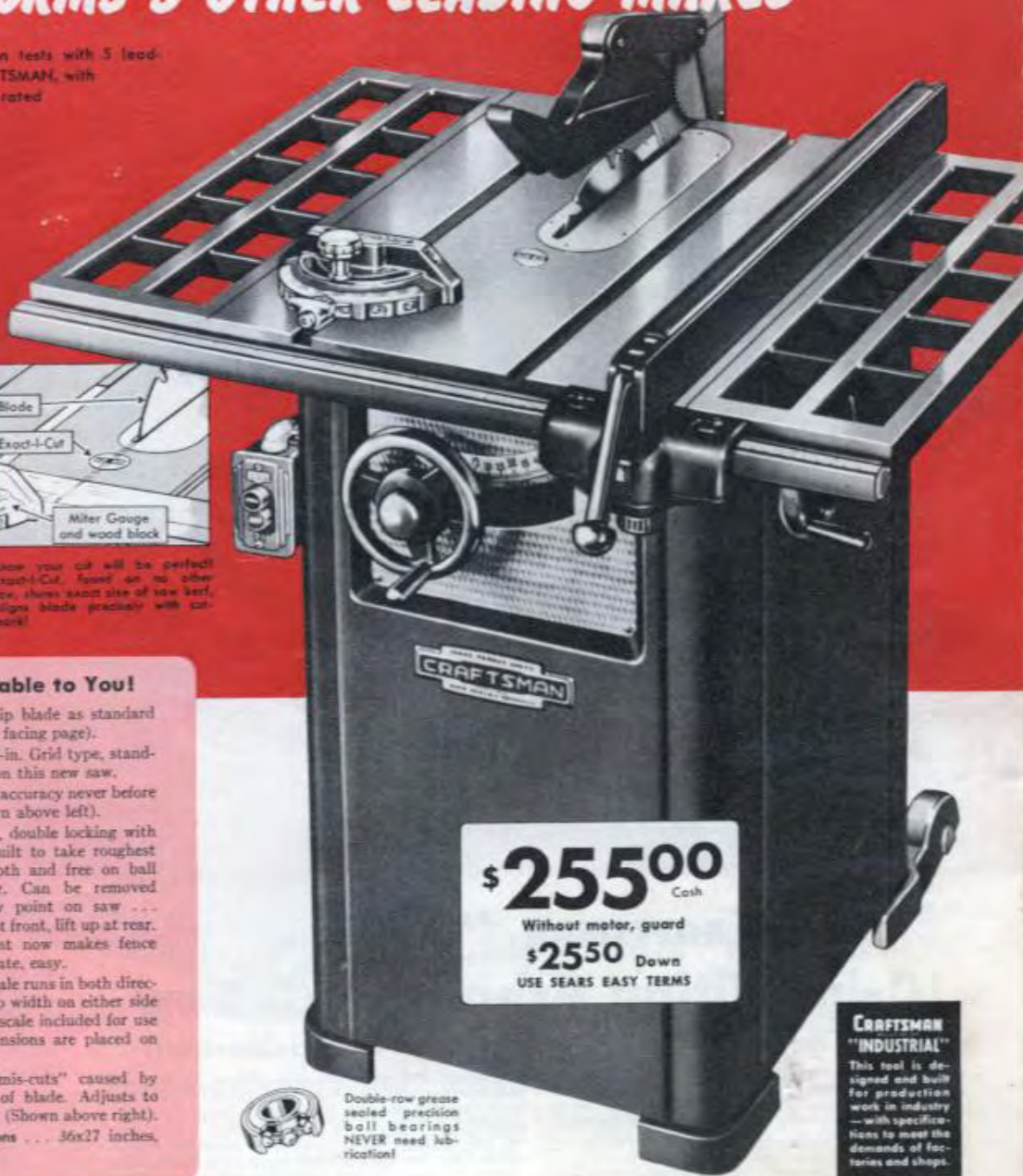
Die cast, self-indexing miter gauge has gripped face; "hypodynamic" type grip controls plunger for uniform accuracy. Sets at 45 and 90 degrees.
